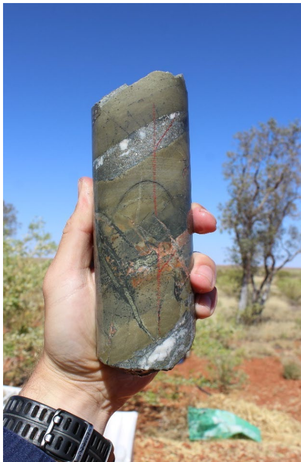
Photo 4 - Example of altered and veined siltstone containing quartz carbonate-pyrite with chalcopyrite veining ~280.5m in ETG0243
