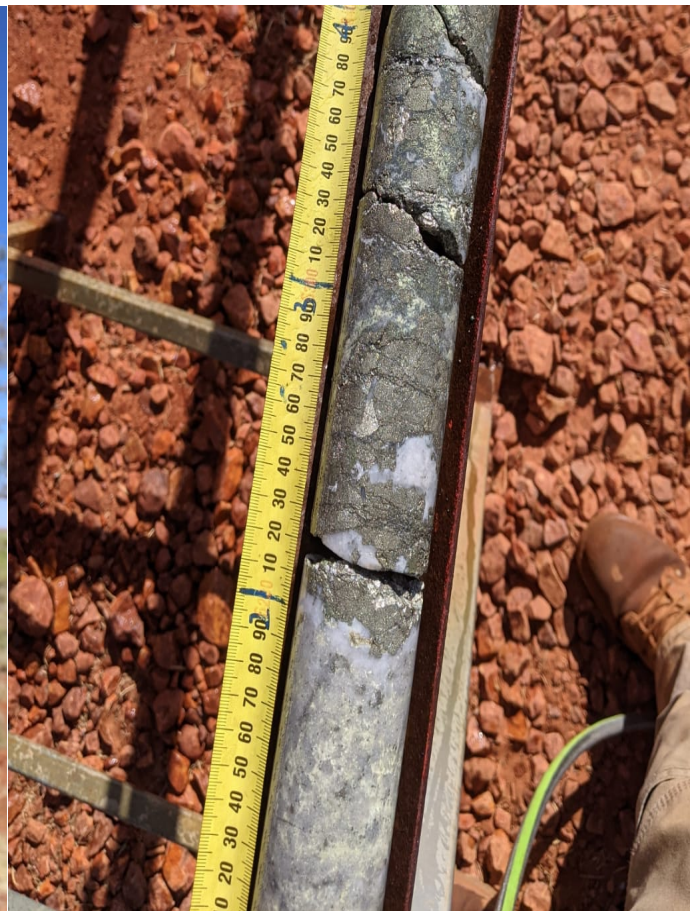
Photo 5 - Example of semi-massive pyrite/chalcopyrite in quartzite unit ~ 347m in ETG0243
