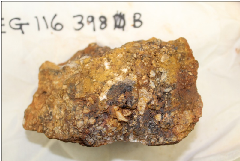
Photo 2. Rock chip sample EG116398B containing 0.5% TREO (including 0.1% \text{Nd}_2\text{O}_3 + \text{Pr}_6\text{O}_{11} ). This sample was taken from an area of outcropping iron altered quartzite north of gravity Anomaly 5.
