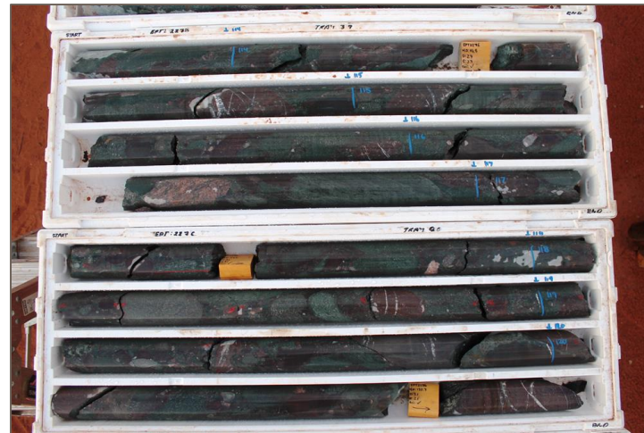
EPT2276 intersected further hematite-altered, polymictic breccia containing blebs of copper sulphide
