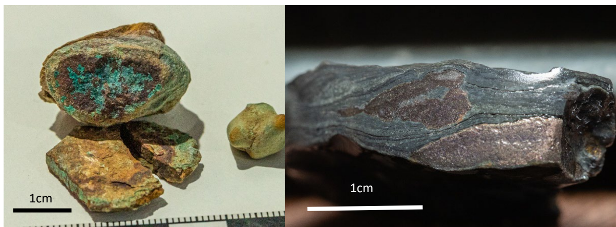
Photo 1 (left) – weathered copper rich nodules collected from surface at Area 1 ( refer Figure 1 ) - containing malachite (interpreted after bornite-chalcopyrite), visual estimate 10% malachite in 2.5cm diameter nodule Photo 2 (right) – primary copper rich nodule from historical drillhole (Mt Skinner DDH3 203.3m) located adjacent to Area 4 ( refer Figure 1 ) containing bornite-chalcopyrite, visual estimate 30% bornite-chalcopyrite over ~1cm width.
