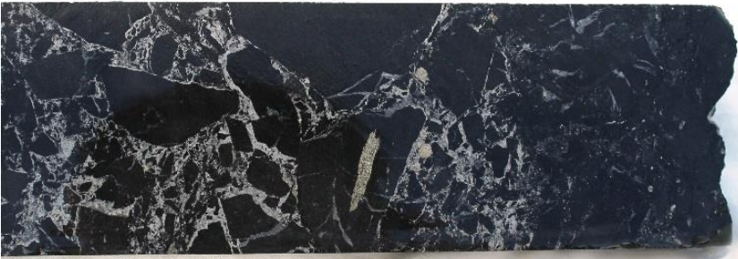
Photo 3: Millennium prospect – EPT2198 (~295m) Sphalerite (light brown) and minor pyrite in brecciated shale. Assaying of this interval returned a grade of 6.6% zinc. Core sample width approx. 50mm
