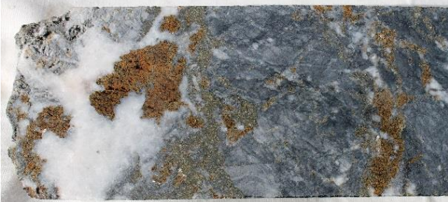
Photo 2: Millennium prospect – EPT2198 (~235.6m) Sphalerite (brown) and pyrite in brecciated carbonate. Assaying of this interval returned a grade of 6.7% zinc. Core sample width approx. 50mm
