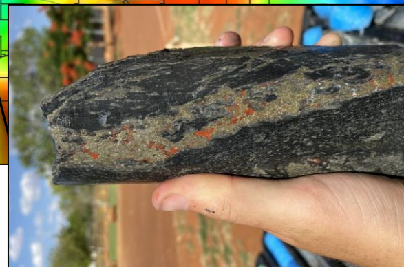
Drill hole NDIBK04 pyrite- chalcopyrite vein 3
