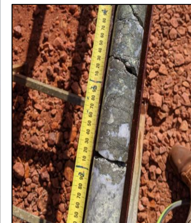
Semi-massive pyrite/chalcopyrite in quartzite unit ~ 347m in ETG0243 • 0.50m @ 0.50g/t Au & 2.70% Cu
