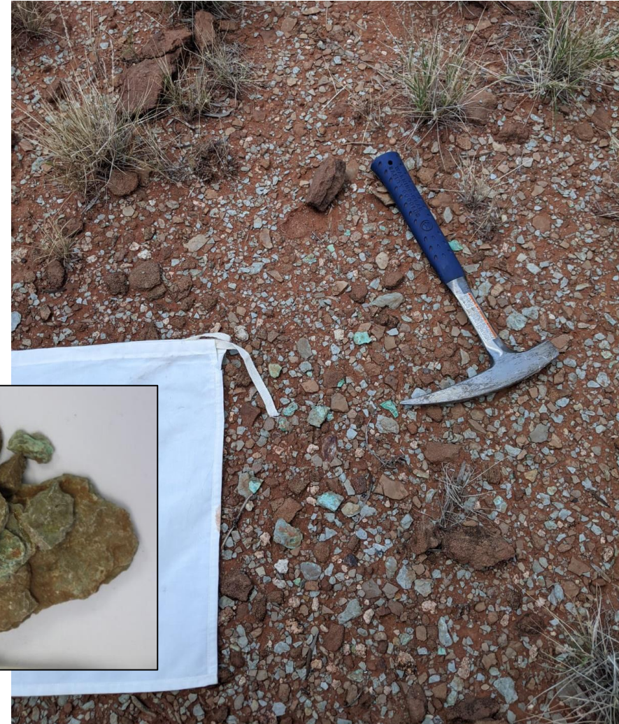
SA0000011 selected sample of surface scree Sandover 5.5% Cu (Area 2)
