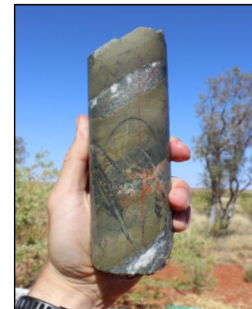
Altered & veined siltstone with quartz carbonate-pyrite with chalcopyrite veining ~280.5m in ETG0243 • 0.23m @ 4.70g/t Au & 1.54% Cu
