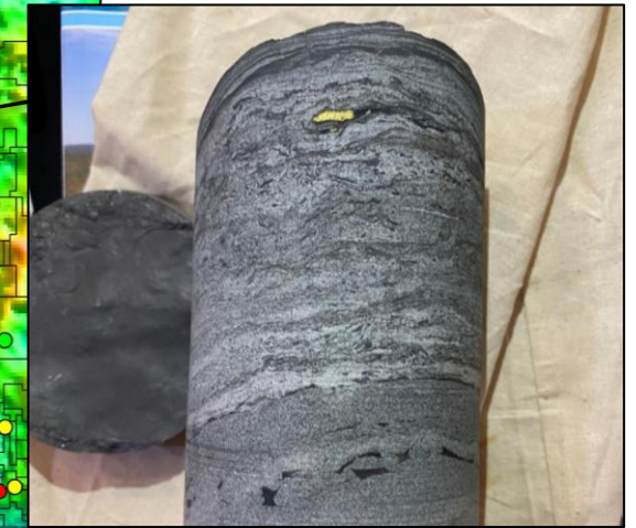
Chalcopyrite contained in a calcareous shale unit within NDI Carrara 4 ~1,617m 4
