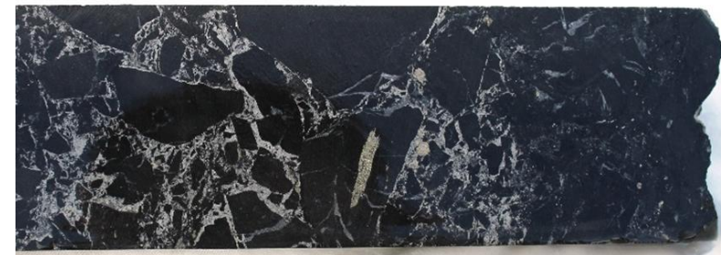
Photo 2: Millennium prospect – EPT2198 (~295m) Sphalerite (light brown) and minor pyrite in brecciated shale - 6.6% Zn core sample width approx. 50mm
