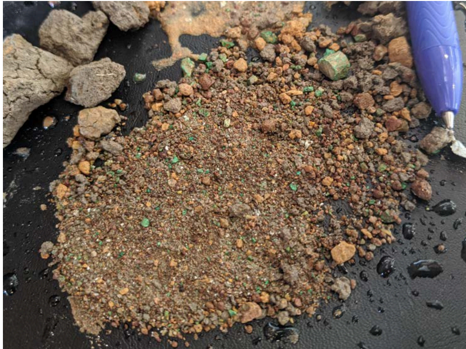
Photo 1 – Copper Carbonate (Malachite) mineralisation at Jessica: 0-3m from RN28419 – chemical assay 1.5% Cu
