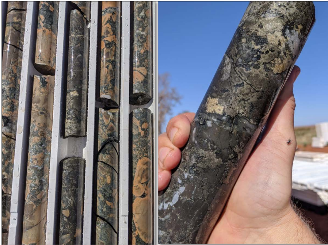
Photo 1 – Brecciated and altered sediments containing disseminated and blebby sulphides in ETG0203 (~185-190m). Photo 2 – Coarse euhedral pyrite and fine pyrite alteration within silicified and brecciated sediment in ETG0203 (~187m). Importantly, the sulphide mineralisation in ETG0203 has a lower chargeability response than the Elsa Prospect.
