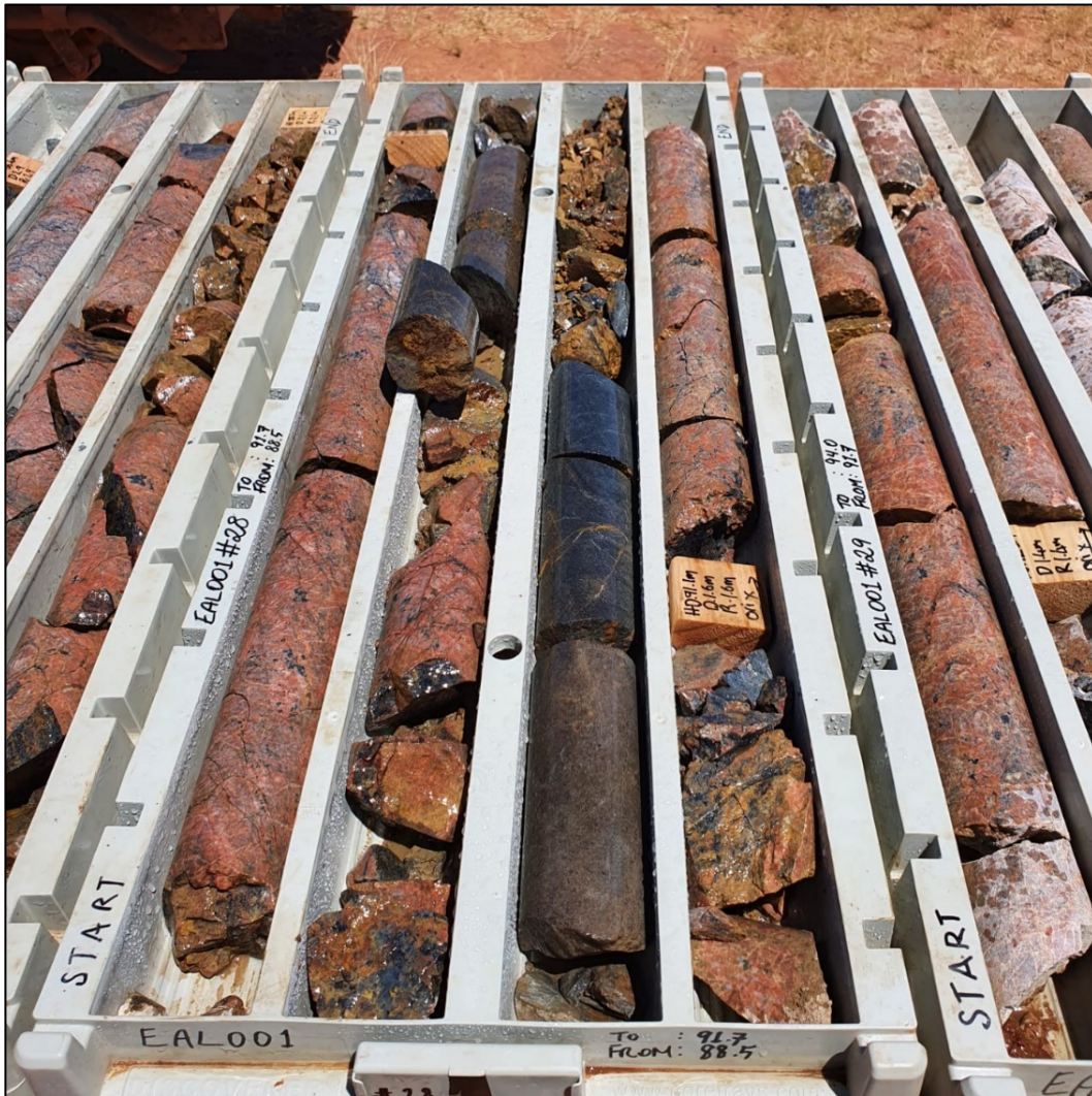
Photo 1 – Hematite altered and fractured, coarse grained granitic rock with narrow mafic intrusive (88.5 - 91.7m)
