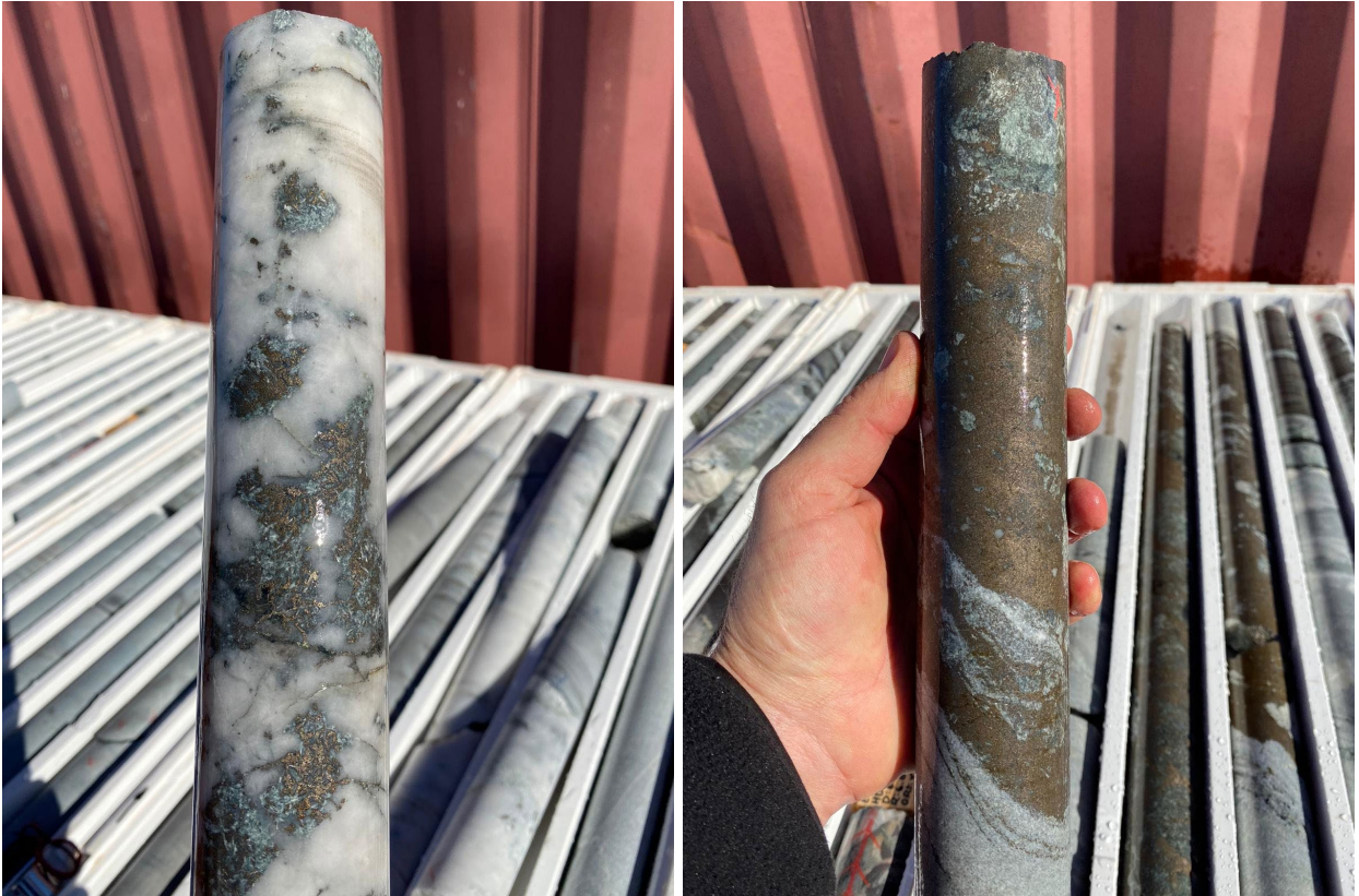
Photos 6 & 7. Examples of quartz sulphide breccia with pyrrhotite at ~320m & ~330m in ETG0241
