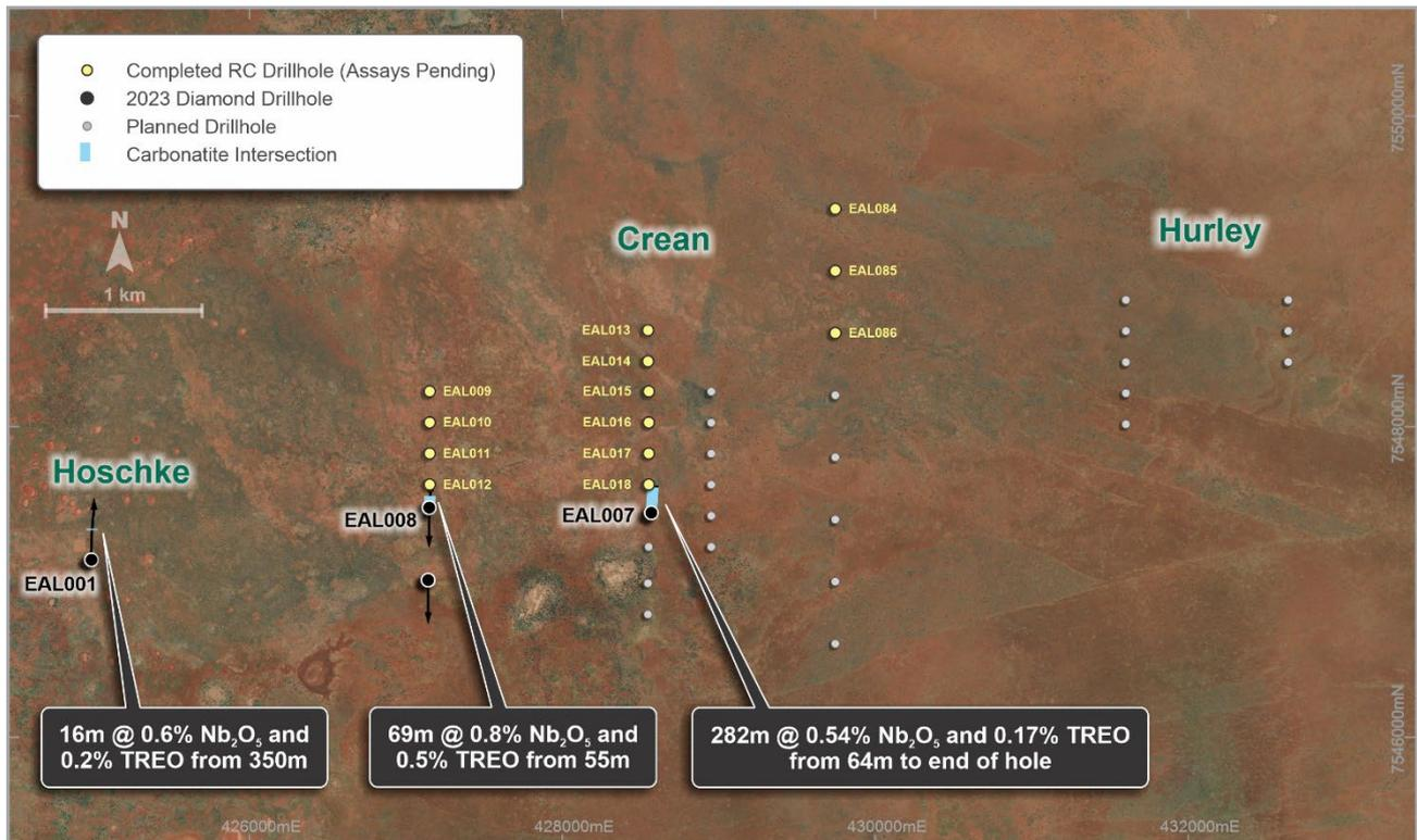
Figure 2 – Aileron diamond drill plan showing the 3 holes (EAL001, EAL008 and EAL007) that intersected carbonatites over 3.5km of strike along the Elephant Island Fault and RC drilling completed and planned.
