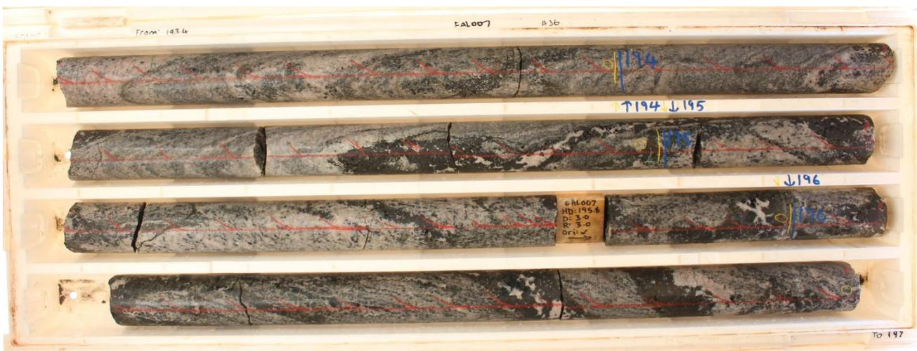
Photo 3: EAL007 Niobium-REE carbonatite 193.4-197m (part of 48.3m @ 1% Nb<sub>2</sub>O<sub>5</sub> from 181.5m)
