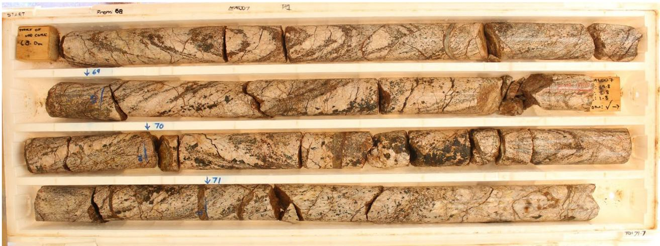
Photo 2: EAL007 Niobium-REE carbonatite 68-71.7m (part of 18.7m @ 1.02% Nb<sub>2</sub>O<sub>5</sub> from 65m)
