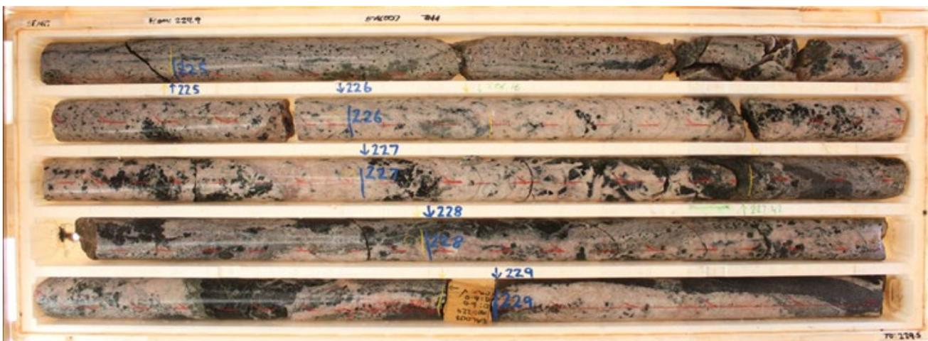
Photo 4: EAL007 Niobium-REE carbonatite 224.9-229.5m (part of 48.3m @ 1% Nb<sub>2</sub>O<sub>5</sub> from 181.5m)
