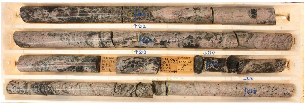
Photo 1: EAL007 Niobium-REE carbonatite 211.6-215.3m (including 4.92m @ 2.16% Nb<sub>2</sub>O<sub>5</sub> from 209.8m)
