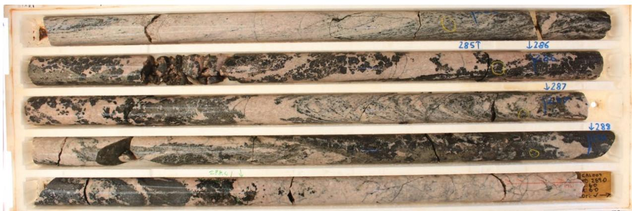
Photo 5: EAL007 Niobium-REE carbonatite 284.4-289m (including 3.41m @ 1.98% Nb<sub>2</sub>O<sub>5</sub> from 285m)
