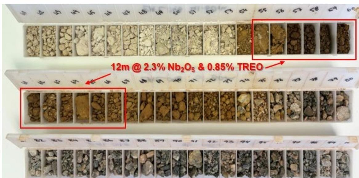
Figure 1 – EAL098 chip trays showing oxide intersection of 12m at 2.3% Nb<sub>2</sub>O<sub>5</sub> from 54m including 2m at 6.3% Nb<sub>2</sub>O<sub>5</sub> and 2.5% TREO from 54m
