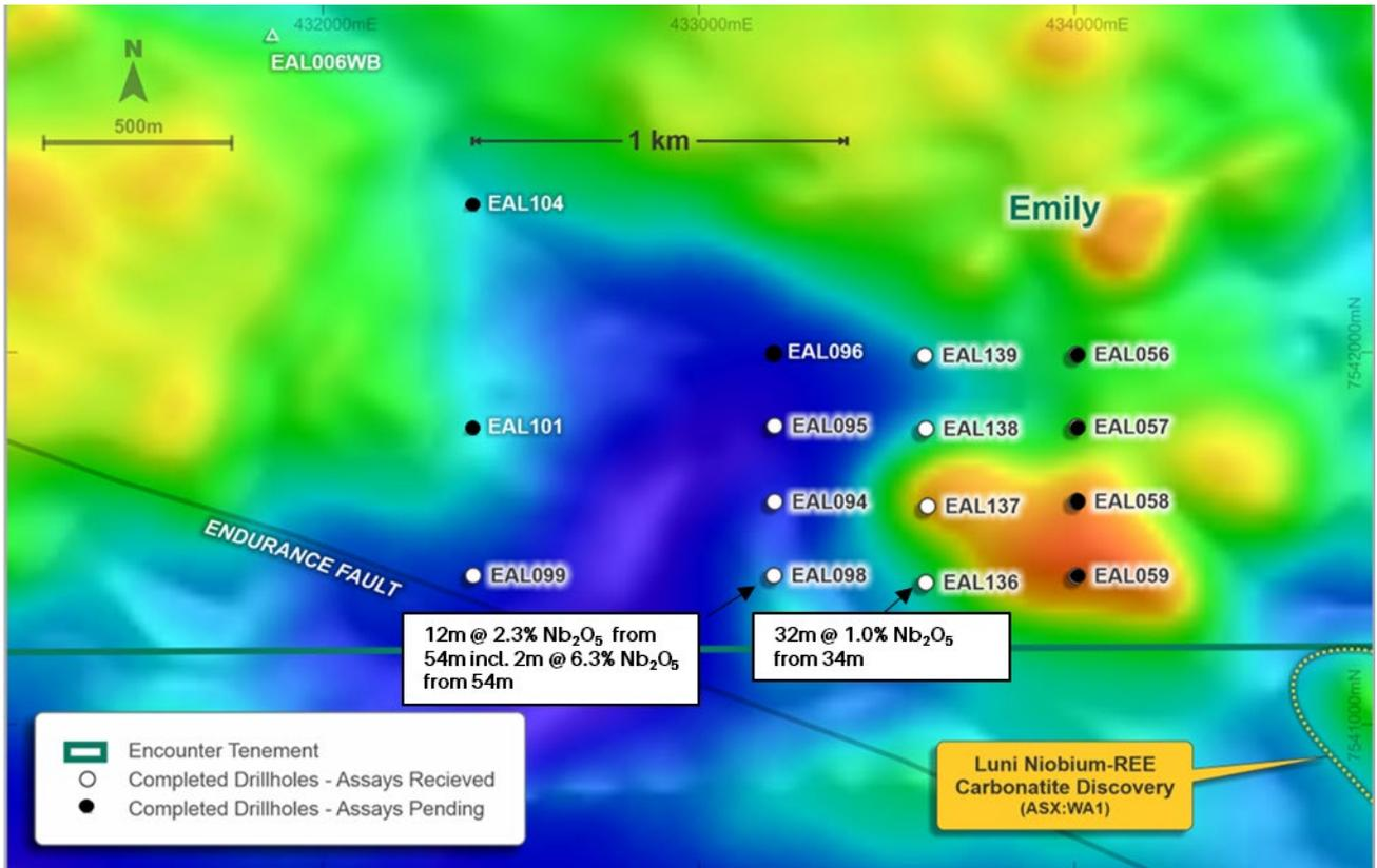
Figure 3 – Emily target drill plan over RTP magnetics
