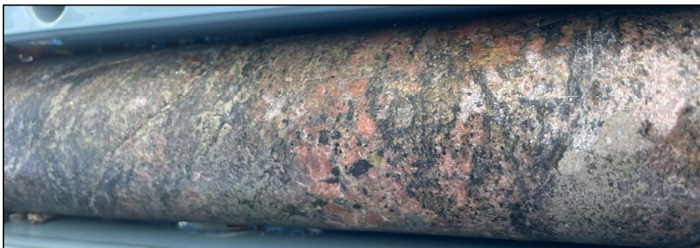
Photo 1 – ESA001 634.4m Strong to intense hydrothermal alteration including chalcopyrite in medium to coarse grained biotite-muscovite granite
