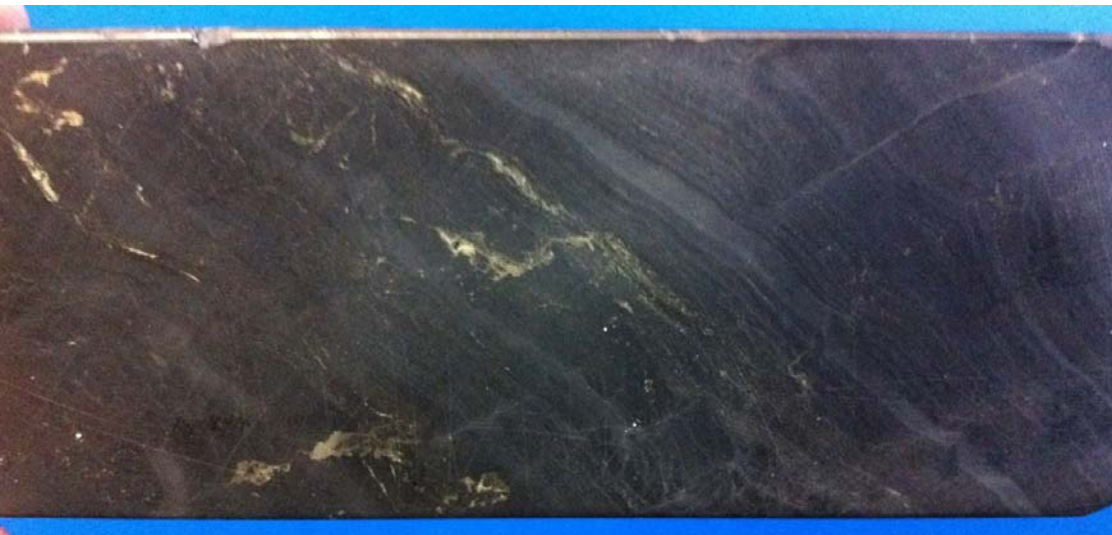
Photo 4: EPT1109 Disseminated chalcopyrite and pyrite (354m) Core diameter approx. 50m
