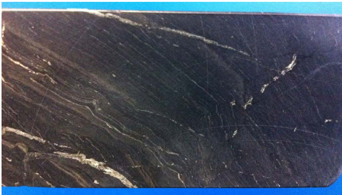
Photo 1: EPT1109 Fine disseminated chalcopyrite and pyrite (244m) Core diameter approx. 60mm
