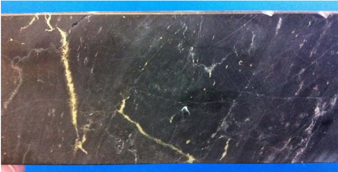
Photo 2: EPT1109 Stringer and disseminated chalcopyrite (288m) Core diameter approx. 60mm
