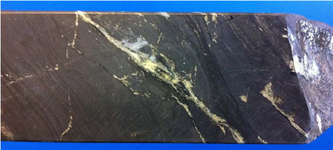
Photo 3: EPT1109 Stringer and disseminated chalcopyrite (305m) Core diameter approx. 50mm
