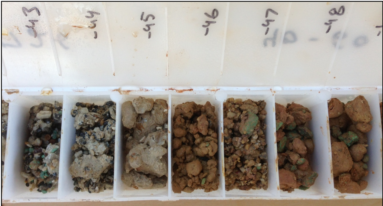
Photo 1 - EPT1726 - Copper mineralisation 43-49m (malachite) within leached clays
