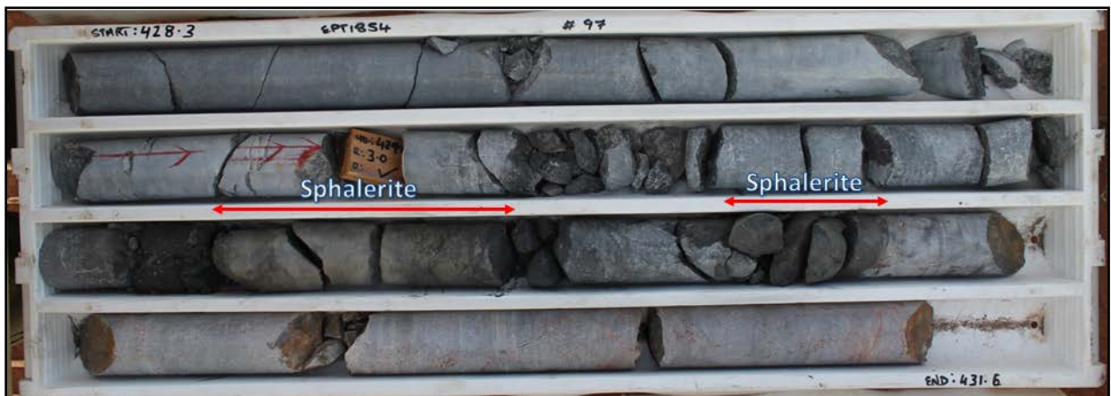
Photo 2 - EPT1854 – ~428.3 to 431.6m – zones of brecciated and laminated massive zinc sulphide mineralisation (Sphalerite)
