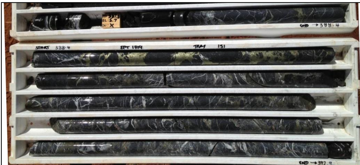
Photo 1 - EPT1719 – ~387.6m to 392.9m – Veined and brecciated carbonate with local massive copper sulphide breccia cement
