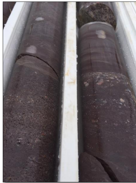
Photo 5: Example of "Red Bed" oxidized sediments EPT2282 ~320m downhole Core width ~60m
