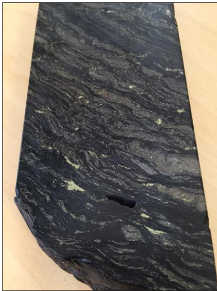
Photo 4: Disseminated chalcopyrite in carbonaceous shale EPT 2282 ~259.5m downhole (1.0%Cu) Core width ~60mm
