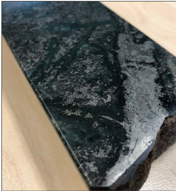
Photo 1 (L) – LSPC-3, ~44m. Veins and disseminations of pyrrhotite and minor chalcopyrite within an altered calcareous sediment
