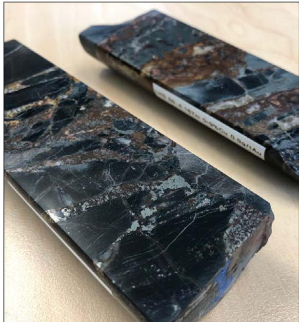
Photo 1 (L) – LSPC-3, ~44m. Veins and disseminations of pyrrhotite and minor chalcopyrite within an altered calcareous sediment
