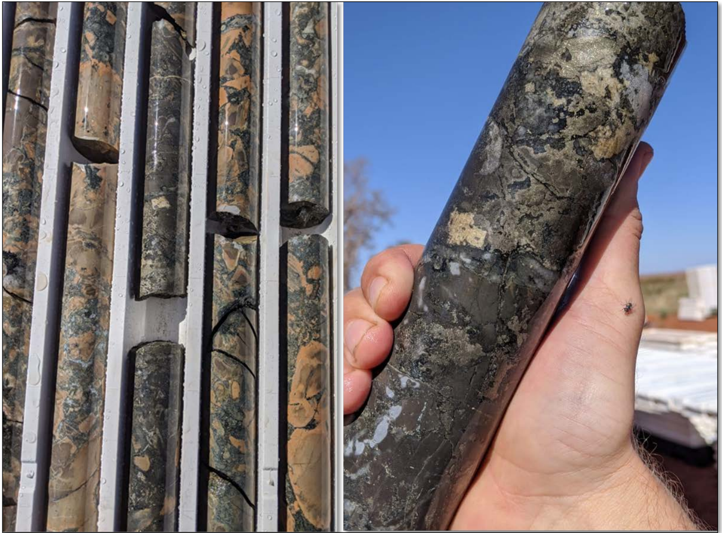
Photos 1&2 ETG0203. Photo 1 (~185-190m) Brecciated and altered sediments containing disseminated and blebby sulphides. Photo 2 (~187m) Coarse euhedral pyrite and fine pyrite alteration within silicified and brecciated sediment
