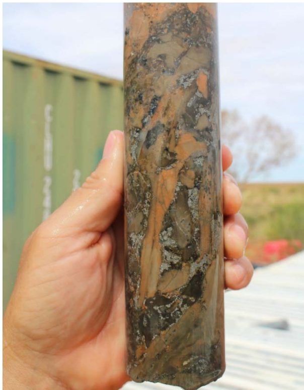
Photo 2 ETG0204. (~315m) Coarse sulphides within brecciated and altered sediments – the silver coloured sulphide mineral is arsenopyrite
