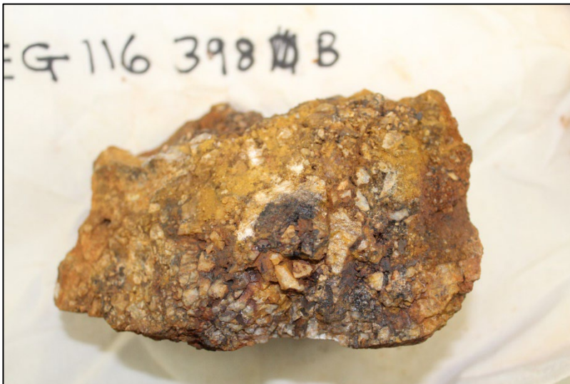
Photo 1. Rock chip sample EG116398B containing 0.5% TREO (including 0.1% Nd 2 O 3 +Pr 6 O 11 ). This sample was taken from an area of outcropping iron altered quartzite north of gravity Anomaly 5.
