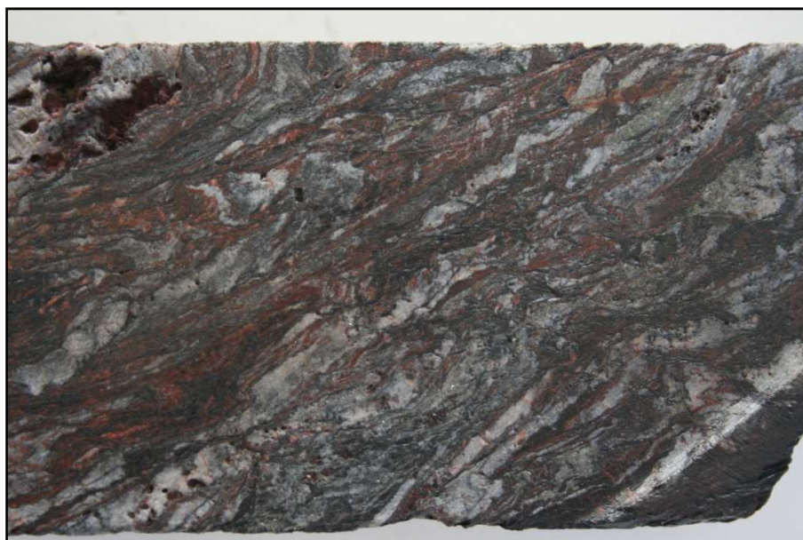
Photo 2 – EPT 574 Haematite-carbonate-pyrite altered black shale at 138m
