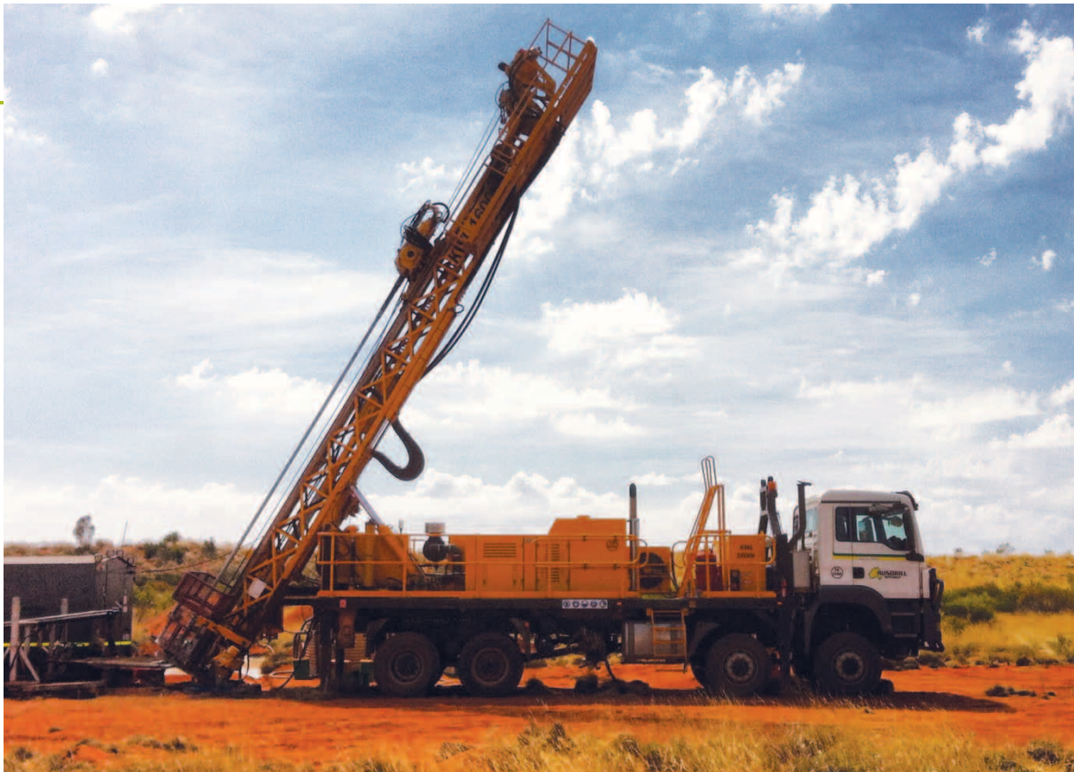
Diamond drill rig at T4
