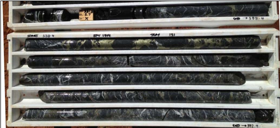
Photo 2. EPT1719 ~387.6m to 392.9m. Veined and brecciated carbonate with local massive copper sulphide breccia cement
