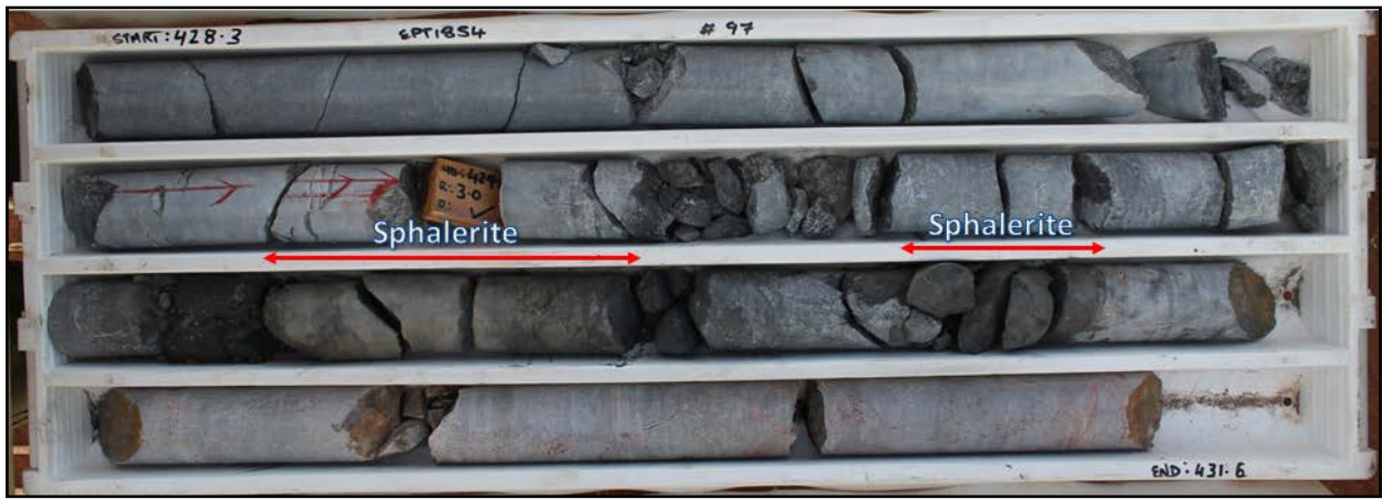
Photo 4 - EPT1854 – ~428.3 to 431.6m – 0.3m and 0.1m wide zones of brecciated and laminated massive zinc sulphide mineralisation
