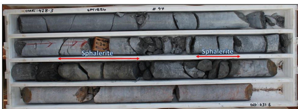
Photo 3 - EPT1854 – ~428.3 to 431.6m – 0.3m and 0.1m wide zones of brecciated and laminated massive zinc sulphide mineralisation.
