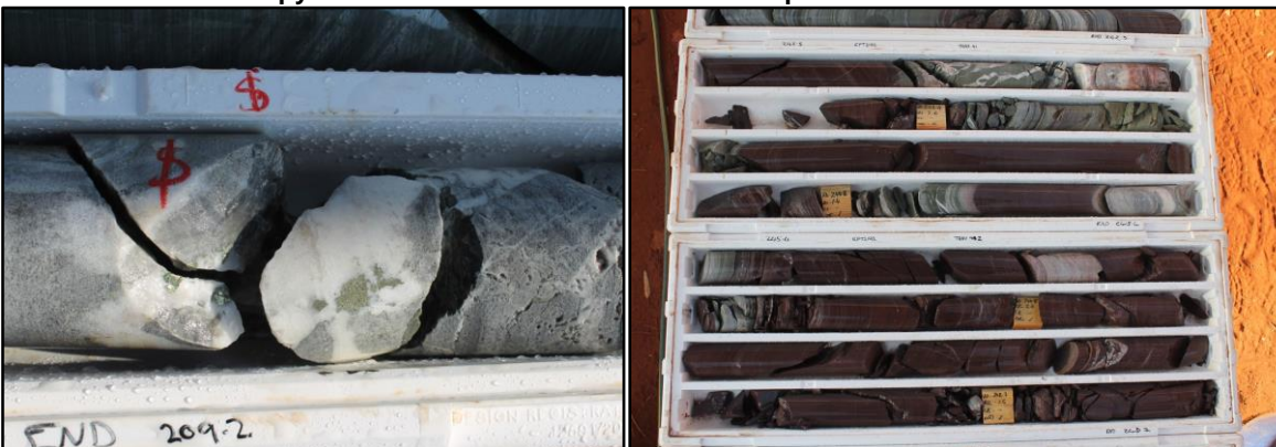
Photo 4 – Chalcopyrite mineralisation from the Moby Dick Prospect at Fishhook ~209m
