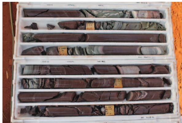
Photo 7: Strong 'red-rock' altered sediments from the Moby Dick Prospect at Fishhook 242-248m
