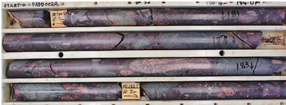
Photo 8: PADD002A 180.4m to 184.0m – Hematite altered, polymictic breccia containing clasts of felsic porphyry, gneissic and mafic igneous rocks
