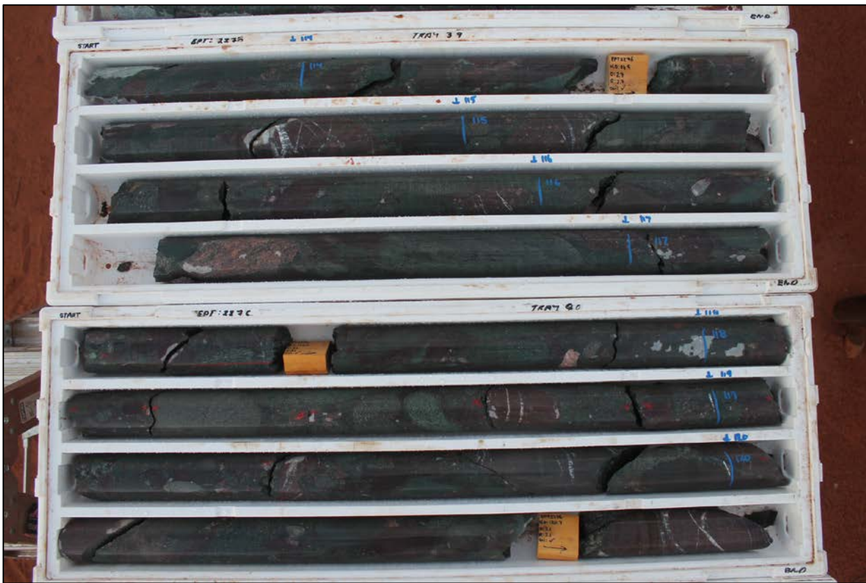
Photo 1: EPT2276 113.7m to 121.0m – Hematite-altered, polymictic breccia containing clasts of felsic porphyry, gneiss and mafic igneous rocks
