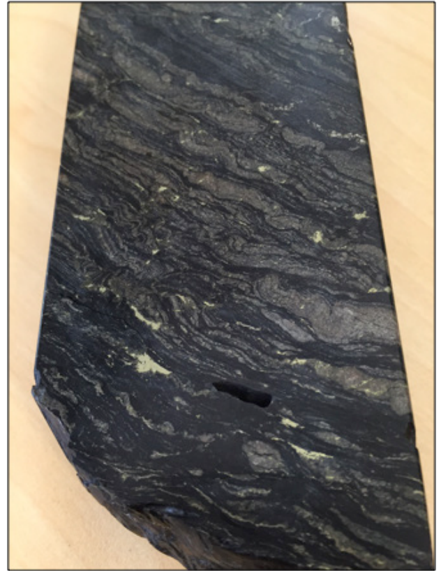
Photo 1: Disseminated chalcopyrite in carbonaceous shale EPT2282 ~259.5m downhole (1.0%Cu) Core width ~60mm
