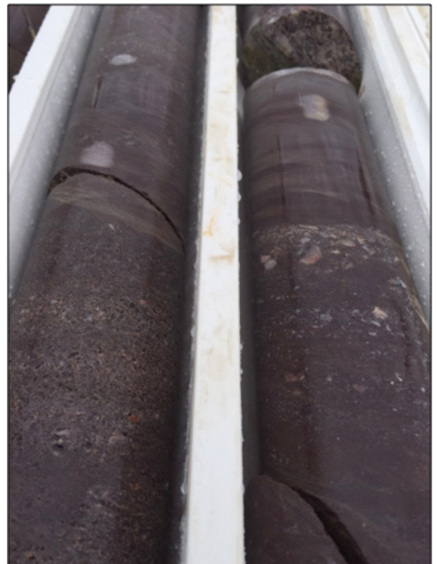
Photo 2: Example of “Red Bed” oxidized sediments EPT2282 ~320m downhole Core width ~60mm
