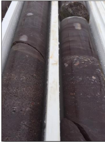
Photo 3: Example of “Red Bed” oxidized sediments EPT2282 ~320m downhole Core width ~60m
