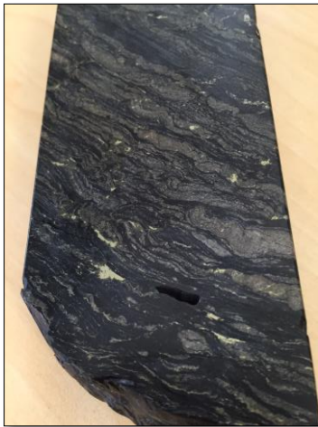
Photo 2: Disseminated chalcopyrite in carbonaceous shale EPT 2282 ~259.5m downhole (1.0%Cu) Core width ~60mm
