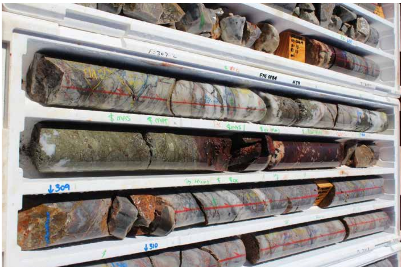
Photo 1 – Drill core from ETG0184 at Telfer West from approximately 307-310m - silicified and fractured quartzite with multiple quartz stockwork style veins containing pyrite and arsenopyrite
