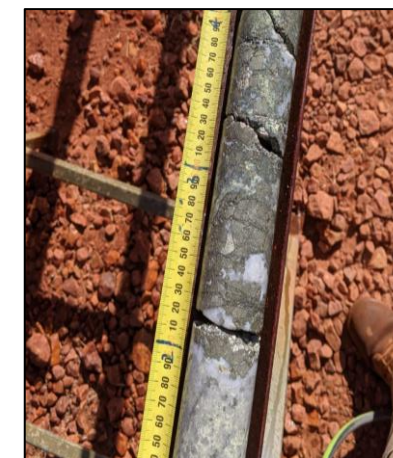
Semi-massive pyrite/chalcopyrite in quartzite unit ~ 347m in ETG0243
