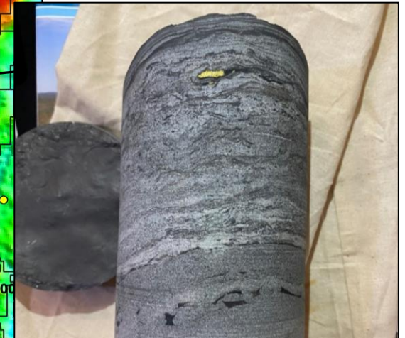
Chalcopyrite contained in a calcareous shale unit within NDI Carrara 4
