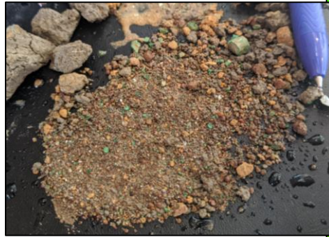
Copper Carbonate (Malachite) 0-3m from RN28419 – chemical assay 1.5% Cu 1
