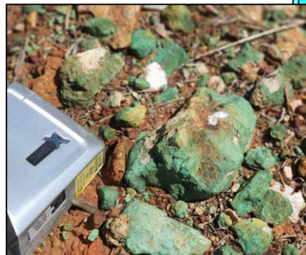
Copper Carbonate (Malachite) 0-3m from RN28419 – chemical assay 1.5% Cu 1
