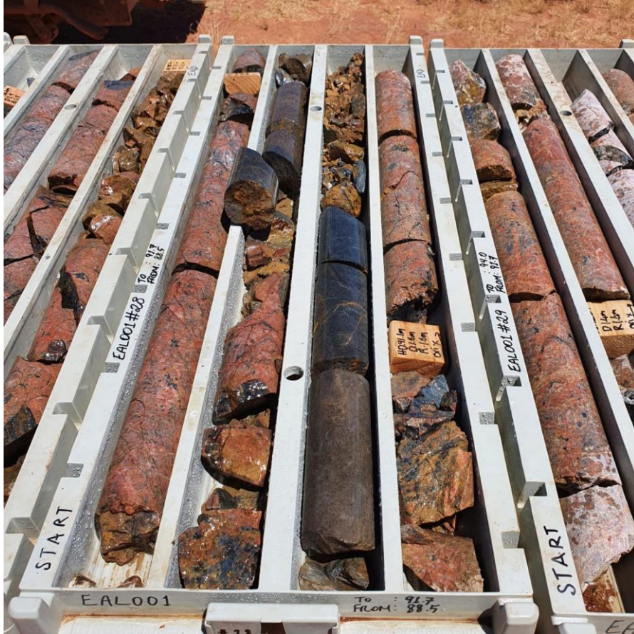
EAL001 - Hematite altered and fractured, coarse grained granitic rock with narrow mafic intrusive (88.5 - 91.7m)
