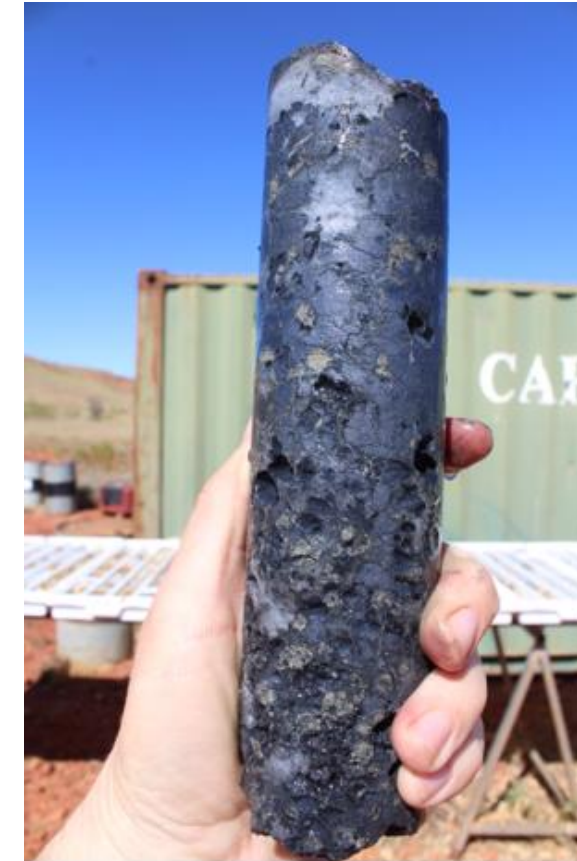
Semi-massive pyrite – chalcocite mineralisation drilled from 409.1 to 410.6m in ETG0226.
