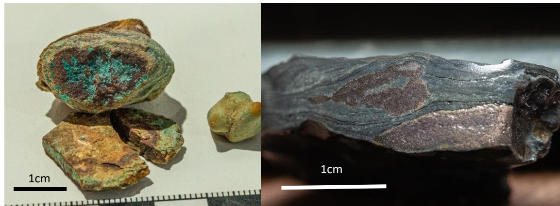
Photo 1- weathered copper rich nodules collected from surface at Area 1 - containing malachite (interpreted after bornite-chalcopyrite)
