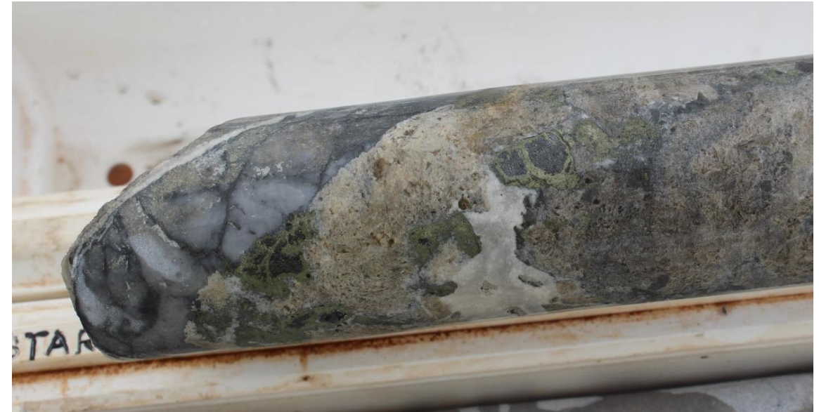
New style of mineralisation intersected at Dune. Epithermal vein containing tetrahedrite which graded 268g/t silver and 2.5% copper at ~617m in ETG0244
