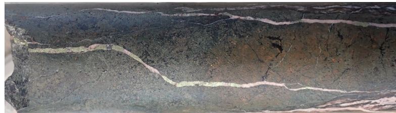
Top – Z23DD002 – Chalcopyrite in quartz-carbonate veins (3.2m estimated 0.25% chalcopyrite from 664.55m) Bottom – Z23DD001 – Bornite-chalcopyrite in chlorite quartz-carbonate vein ~457.3m
