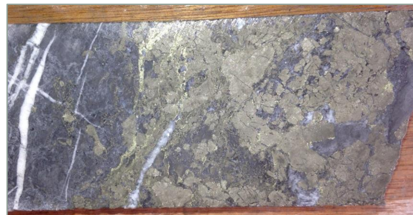
EPT1716 – ~120m - Carbonate with abundant coarse pyrite and with chalcopyrite intergrowths
