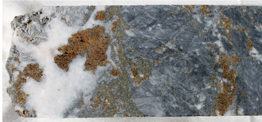
Photo 1: Millennium prospect – EPT2198 (~235.6m) Sphalerite (brown) and pyrite in brecciated carbonate core sample width approx. 50mm
