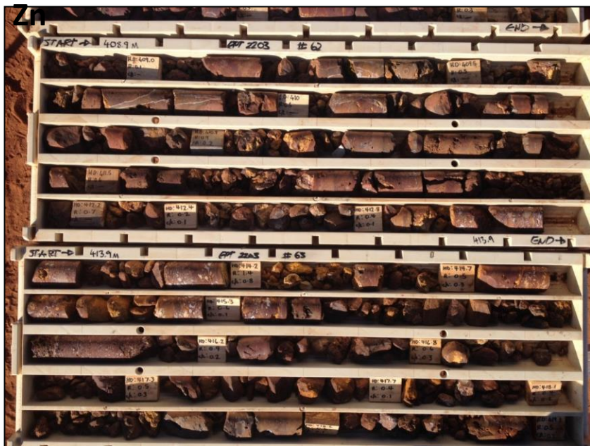
Thick gossan intersections - 70m @ 2.3%
